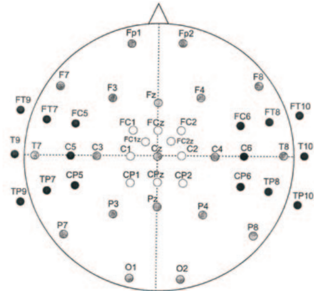
Figure 1. Electrode Configuration for Cortical Array. Shaded electrodes adhere to the International 10/20 system; white electrodes are represented in higher density in region of SMA; black electrodes are represented in higher density overlying the lateral motor cortices.
